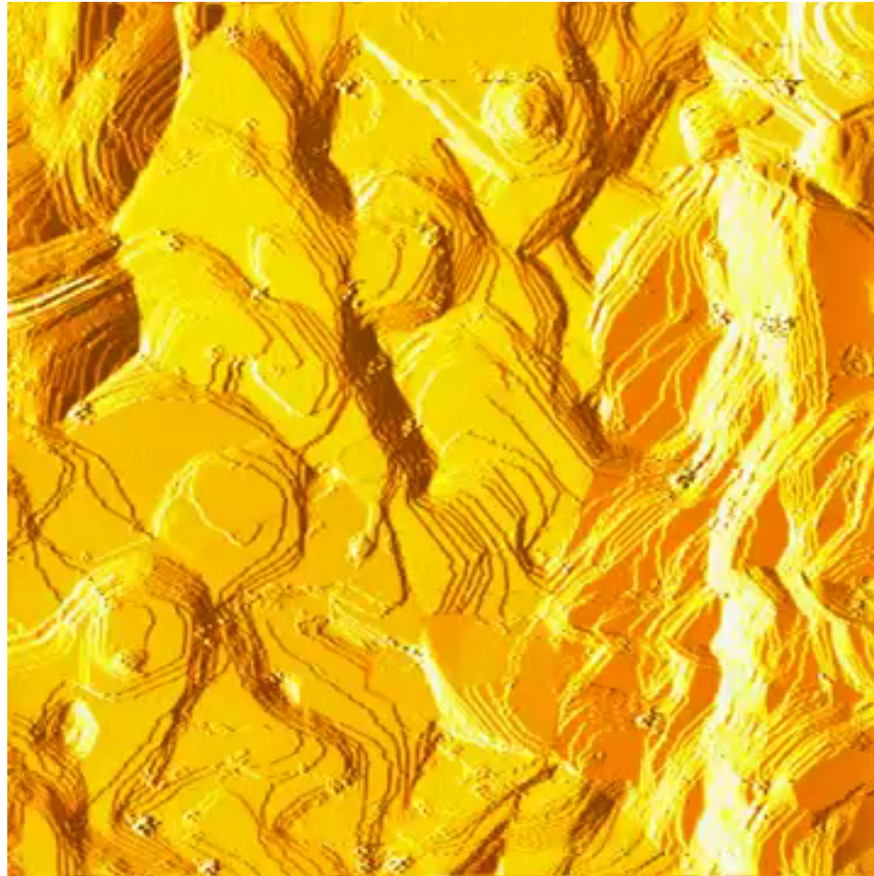
In Situ Real time observation of thin film deposition: Growth of a Polycrystalline film
