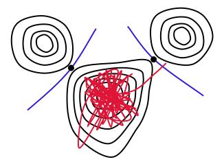
**Fig. 1.** Contour plot of the potential energy surface for an energy-barrier-limited infrequent-event system. After many vibrational periods, the trajectory finds a way out of the initial basin, passing a ridgetop into a new state. The dots indicate saddle points.
