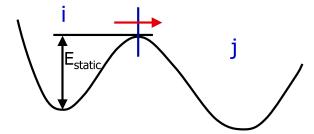
**Fig. 3.** Illustration of the transition state theory rate constant. The unimolecular rate constant for escape from state i to state j,  $k_{ij}$ , is given by the equilibrium outgoing flux through the dividing surface separating the states.
