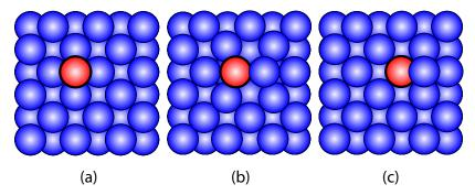
**Fig. 6.** Exchange mechanism for adatom on fcc(100) surface. (a) initial state; (b) saddle point; (c) final state. This mechanism, unknown until 1990 [52], is the dominant diffusion pathway for some fcc metals, including Al, Pt, and Ir.
