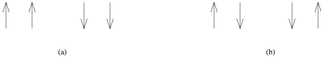
Figure 3: Two-spins configurations: (a) There are two aligned spin configurations. The energy of each configuration is \epsilon_{i,j} = -J S_i S_j = -J . (b) There are two configurations in each of which the spins are not aligned. The energy of each configuration is \epsilon_{i,j} = -J S_i S_j = +J .
