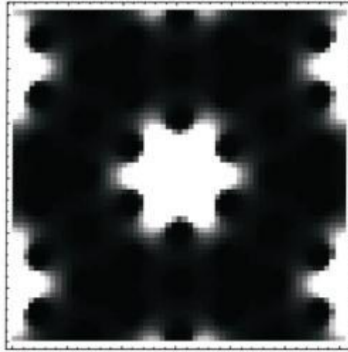
Figure 11: Near field plot of lowest eigenmode ( |\mathcal{E}|^2 ) for a structure of d/a = 0.3 , k_x = 0 , k_y = 0 , k_x = 12.6 \left( \frac{2\pi}{a} \right) , \epsilon_r = 12.25 . 1089 plane waves were used in each direction.
