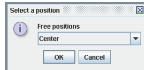
Figure 3.3: A layout manager determines the position of an object in a container. Available positions for the border layout are Center , Up , Down , Left , and Right .
