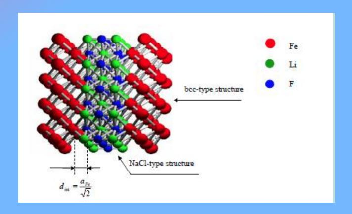
Due to open structure of LiF, to fulfil ASA space filling requirement two empty spheres (ES) at interstices positions at Fe/LiF (100) interface; Fe located atop of F
