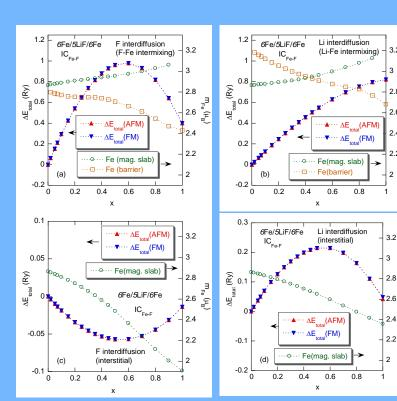
F-Fe intermixing: Fe interdiffusion:  $E_{tot}$  (AFM, FM): increase up to x = 0.6 and then decrease Li-Fe intermixing: Li interdiffusion:  $E_{tot}$  (AFM, FM): increases
