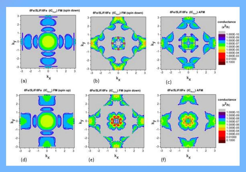
Majority-spin FM conductances: free electron-like with broad peak and large transmission maximum at  $\overline{\Gamma}$  point. Conductance determined by  $\Delta_1$  states.
